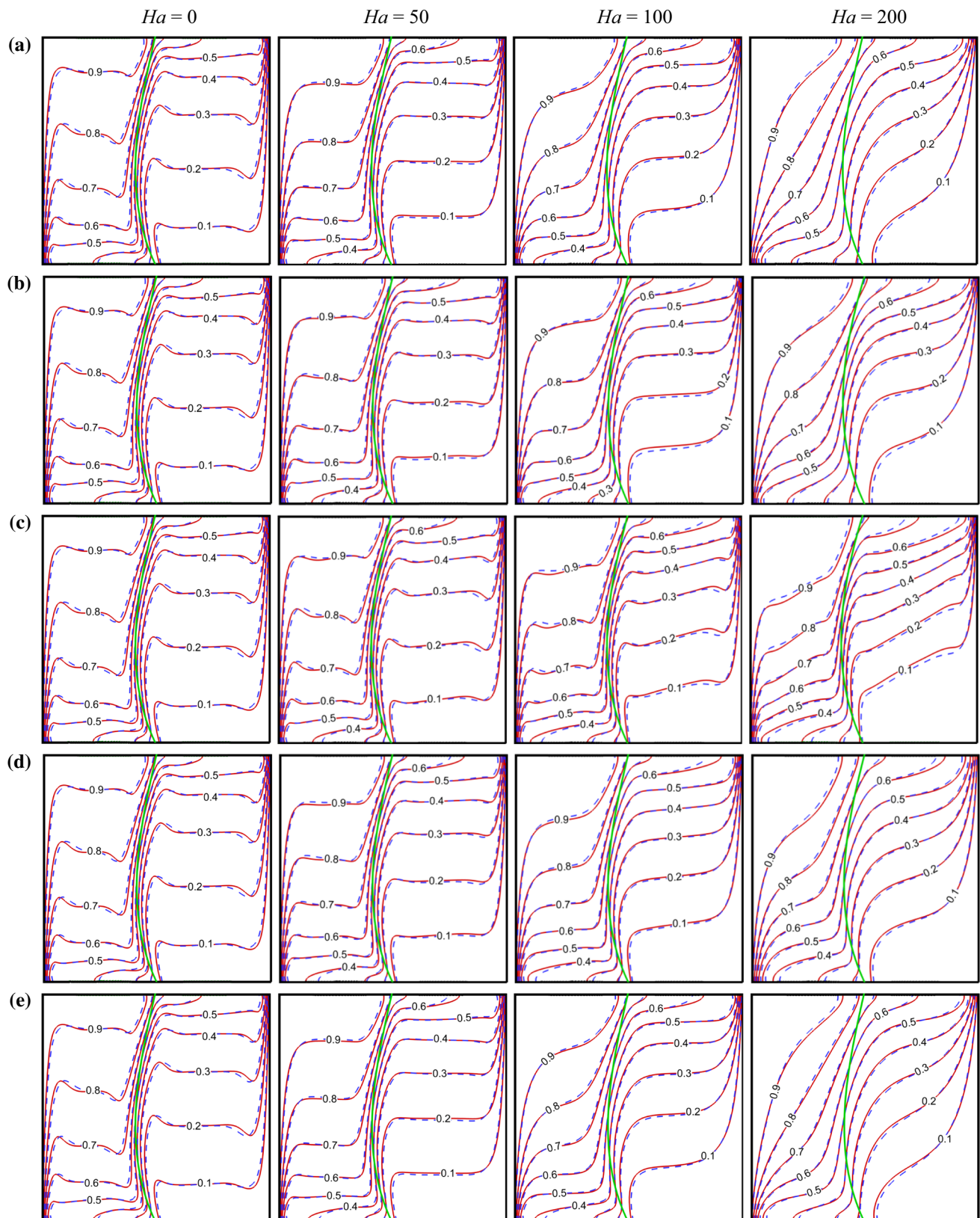
Fig. 14 The isotherms contours of the hybrid nanofluid (dashed lines) and the nanofluid with \text{Al}_2\text{O}_3 nanoparticles (solid lines) for different values of Ha in a \gamma = 0 , b \gamma = 45 , c \gamma = 90 , d \gamma = 135 and e \gamma = 180 for Ra = 10^7 and \phi_{\text{hnf}} = \phi_{\text{Al}_2\text{O}_3} = 2\%
