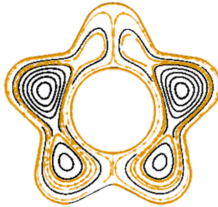
Fig. 5. The obtained streamlines through the current code (black lines) and the data reported in Ghalambaz et al. [52] (brown lines). (For interpretation of the references to colour in this figure legend, the reader is referred to the Web version of this article.)
