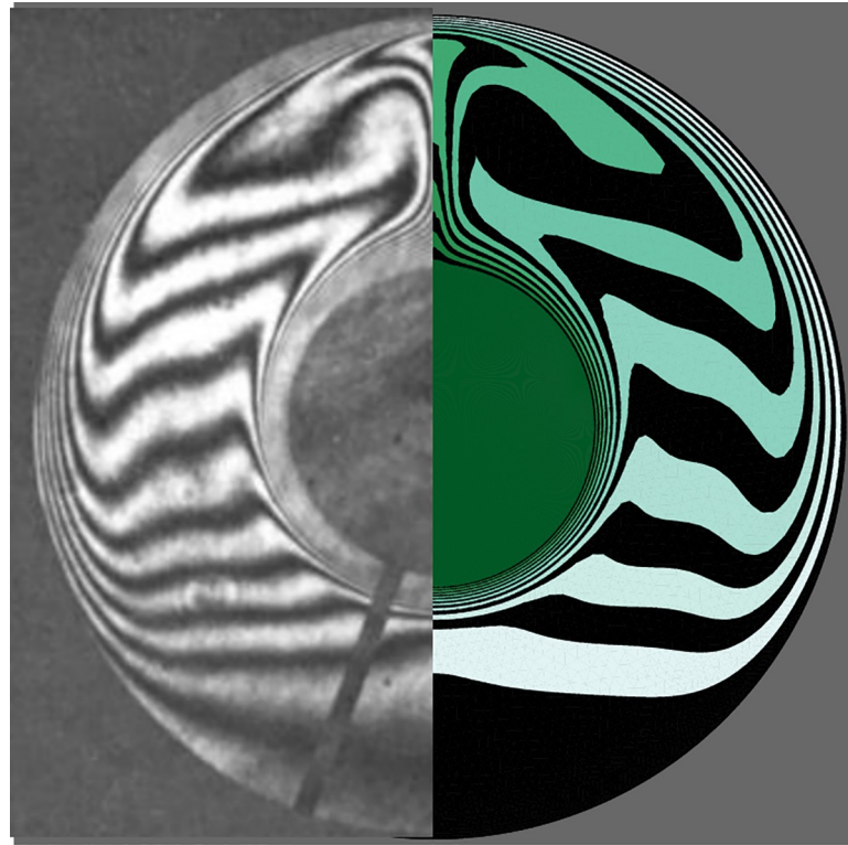
Fig 7. The experimental observations of [53] (right) and the present simulation (left).
